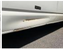
Bumper R, Broken, Replace
