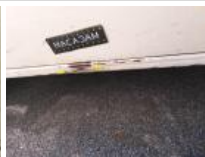
Outside rear-view mirror base L, Scratch(es), Replace
