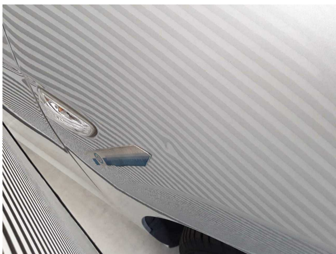
Damage 3: Mudguard - right side: Mudguard - right side - dent(s) - Smooth repair work
