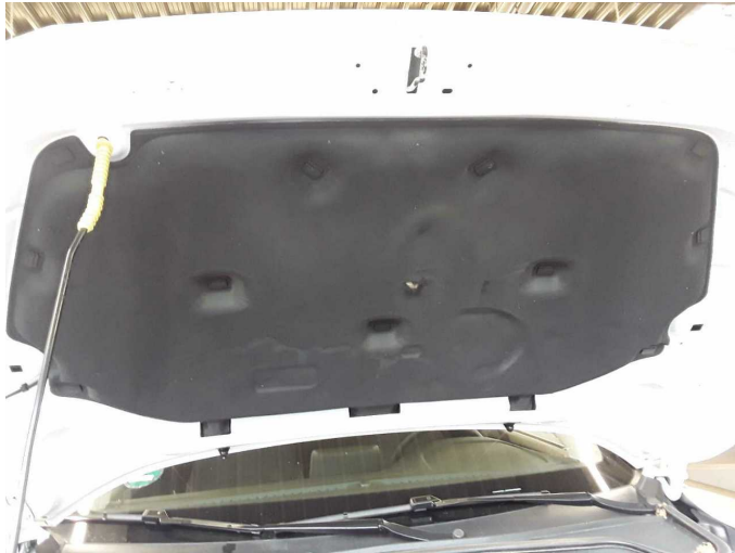
Damage 2: Bonnet: Insulation lining - Damaged - Replace
