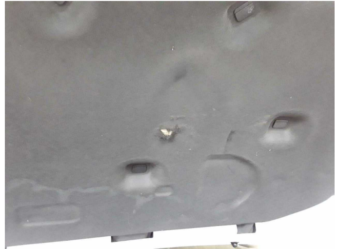
Damage 2: Bonnet: Insulation lining - Damaged - Replace
