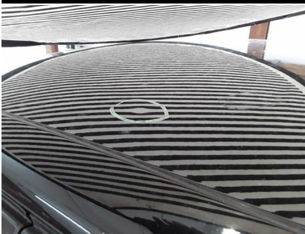
Damage #10: Roof: Roof - dent(s) - Smooth repair work
