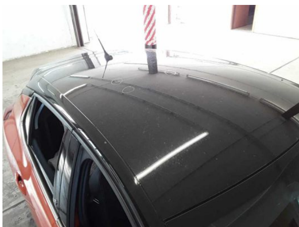
Damage #10: Roof: Roof - dent(s) - Smooth repair work
