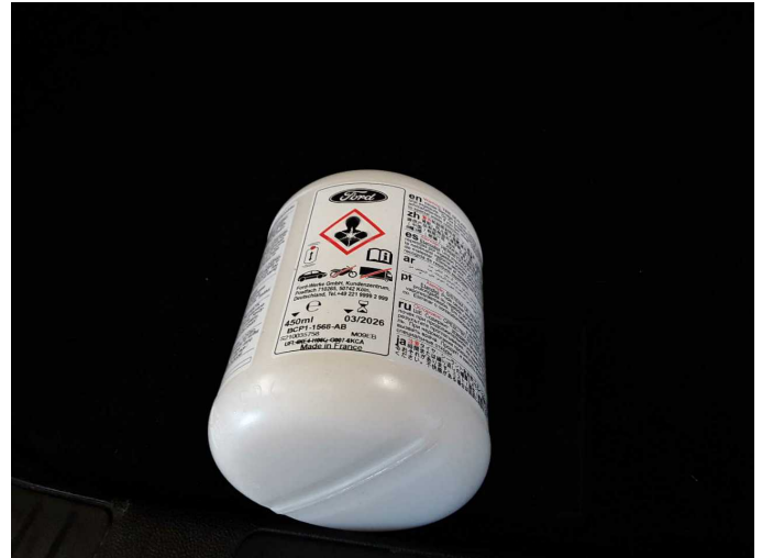
Damage 1: Equipment: Tirefit filler - Expired - Replace
