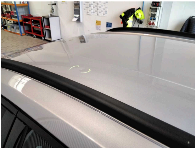
Damage 3: Roof: Roof - dent(s) - Smooth repair work
