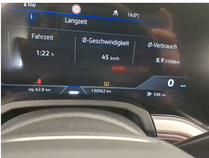
Damage 1: Instrument panel: Indicator light (Reifendruck Kontrollleuchte) - on - Perform diagnosis
