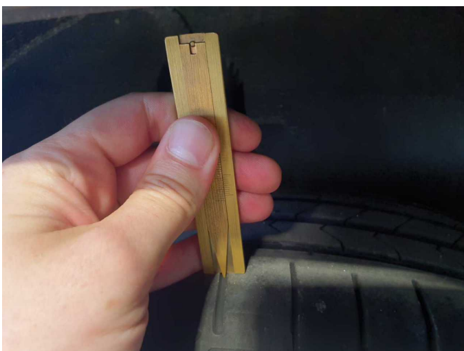
Damage 5: Wheel / tyres: Tyre - rear right side - Worn - Replace
