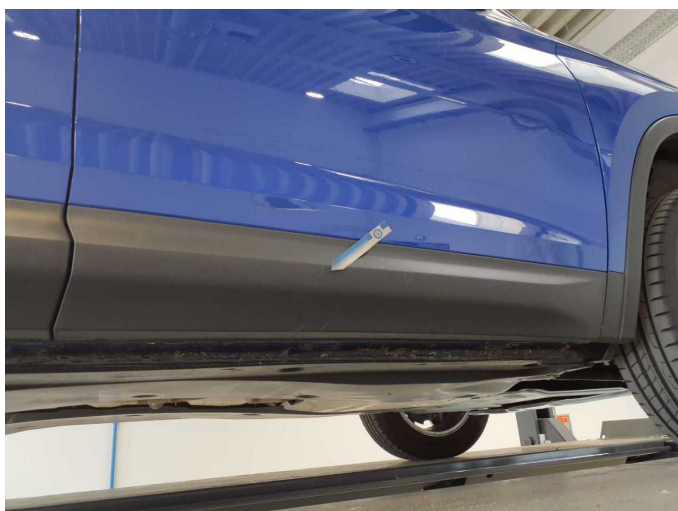
Damage 8: Door - front right side: Brightware - lower - Scratch(es) - Replace
