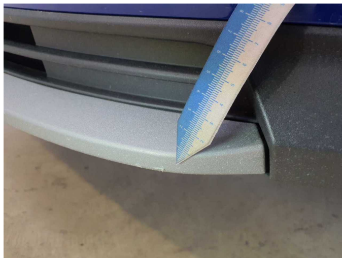
Damage 9: Front bumper: Spoiler - Scratch(es) - Replace
