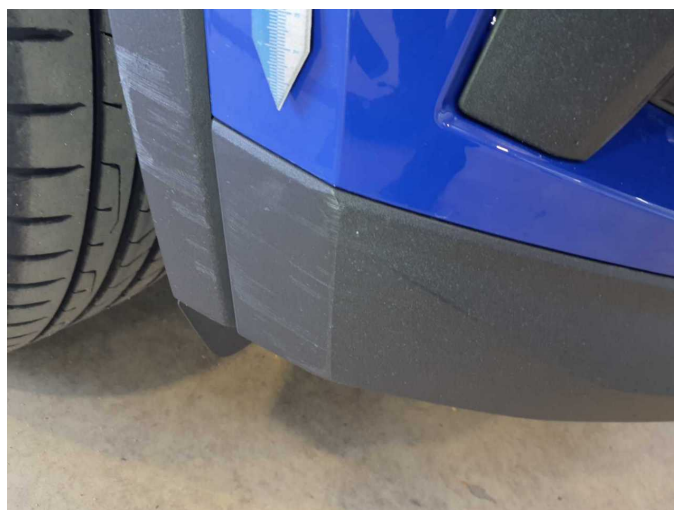
Damage 9: Front bumper: Spoiler - Scratch(es) - Replace
