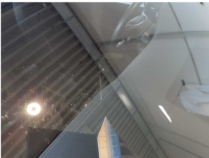
Damage 14: Vehicle glazing: Windscreen - Broken / torn - Replace
