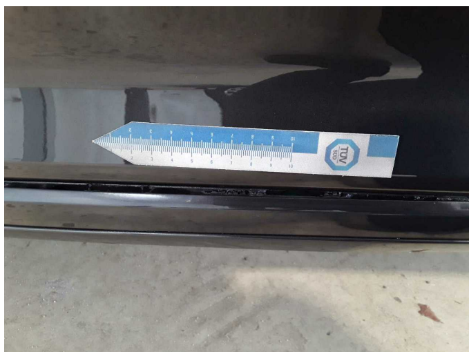
Damage 1: Door - front left side: Brightware - lower - Loose - Un- / install
