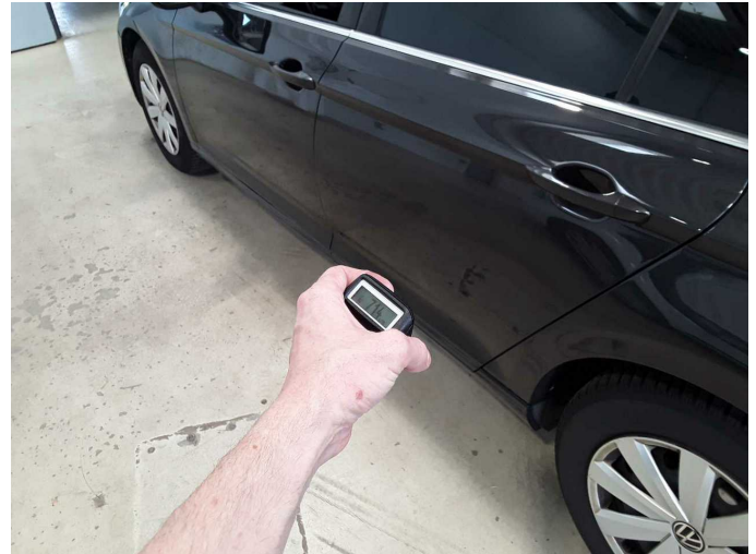
Repainting 2: Door - rear left side
