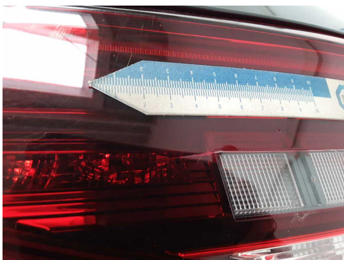
Damage 4: Tail light: Tail lamp - right side (Innen) - Broken / torn - Replace
