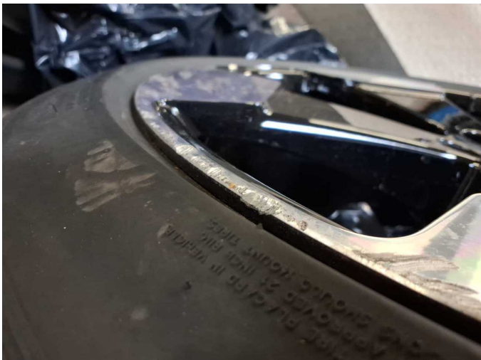
Damage 9: 2nd wheel set: 1 alloy rim (HR, Materialabtrag) - Scratched - Replace
