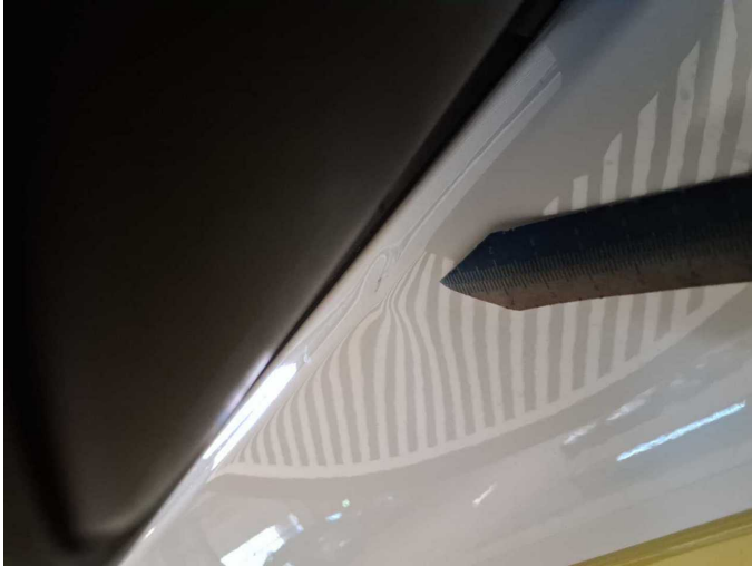
Damage 7: Door - front right side: Door - Deformed - Paint
