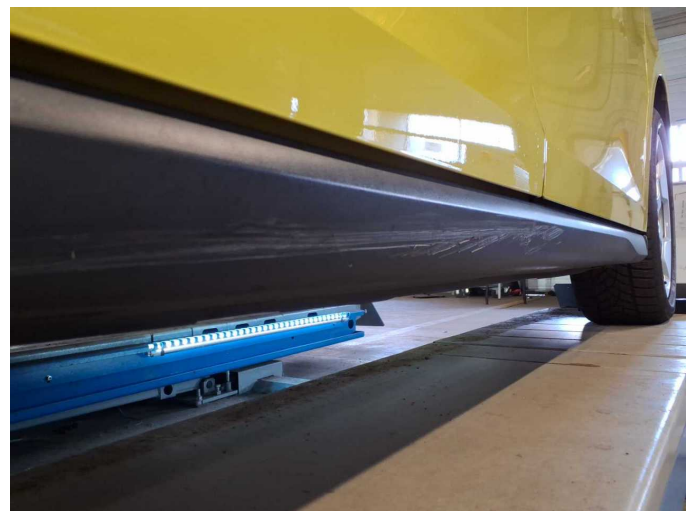
Damage 5: Sill - right side: Trim - Scratched - Replace
