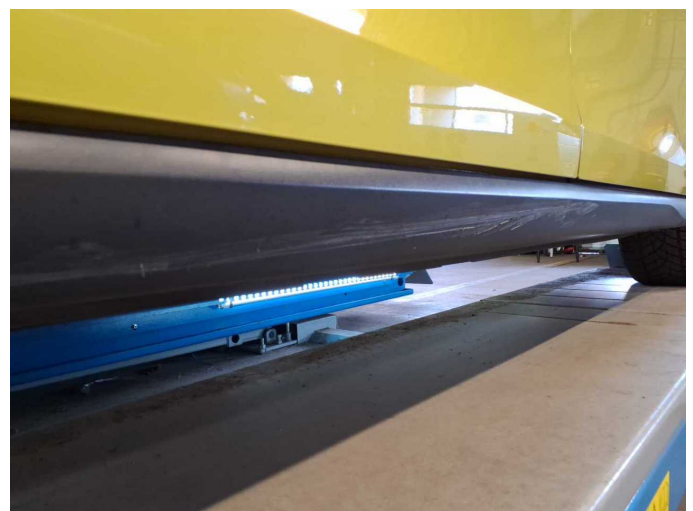
Damage 5: Sill - right side: Trim - Scratched - Replace
