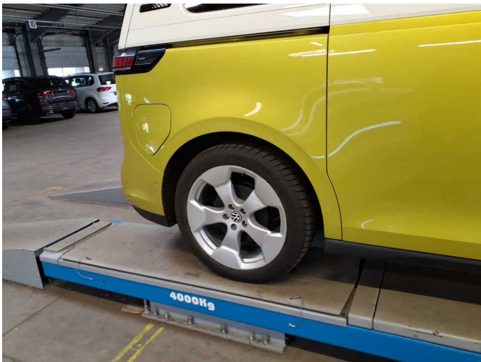
Damage 8: Wheel / tyres: Alloy rim - rear right side (Materialabtrag) - Scratched - Replace
