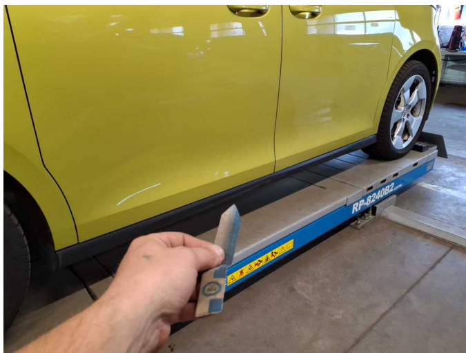
Damage 5: Sill - right side: Trim - Scratched - Replace
