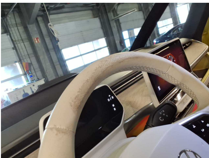
Damage 3: Steering system: Steering wheel - Abrasion - Smart repair
