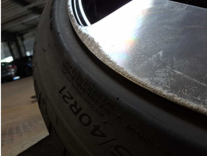
Damage 10: 2nd wheel set: 1 alloy rim (HL, Materialabtrag) - Scratched - Replace
