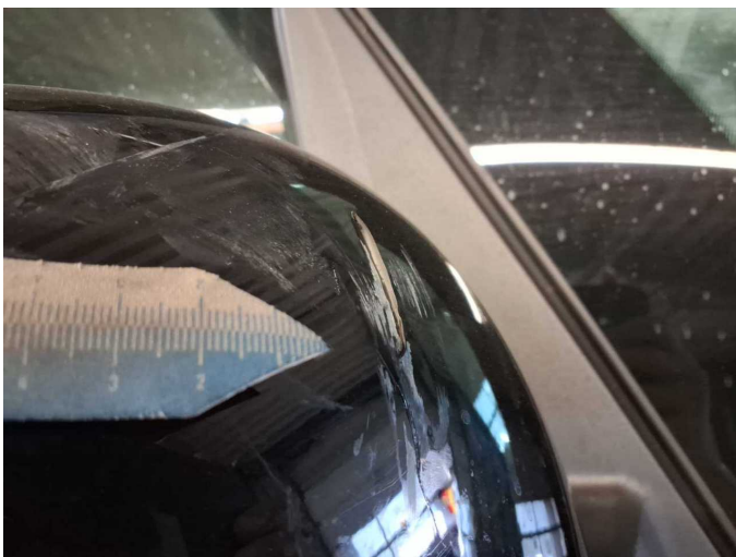
Damage 2: Wing mirror - right side: Cap - Broken / torn - Replace
