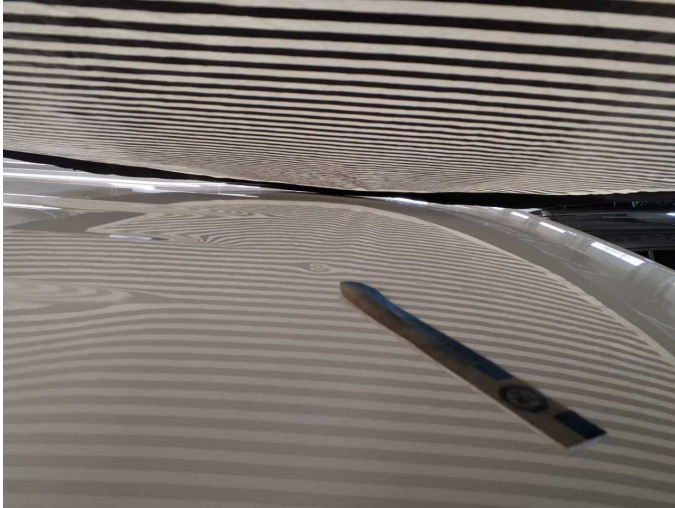
Wear and tear 3: Roof: Roof - dent(s) - No deduction
