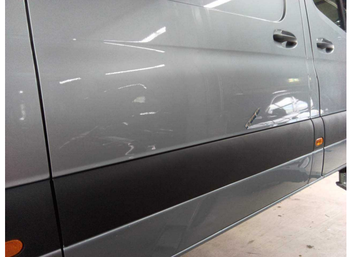
Damage 10: Sliding door, right: Sliding door - Dent / paintcoat damage - Paint
