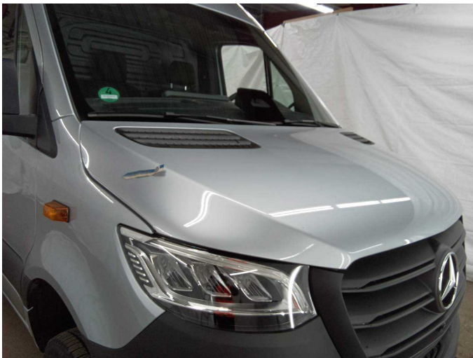
Damage 5: Bonnet: Bonnet - Malposition - Un- / install
