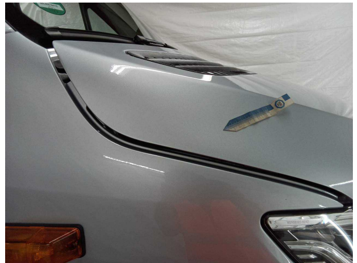
Damage 5: Bonnet: Bonnet - Malposition - Un- / install
