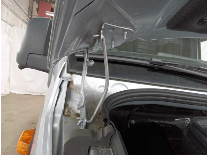
Damage 1: Bonnet: Support - Damaged - Replace
