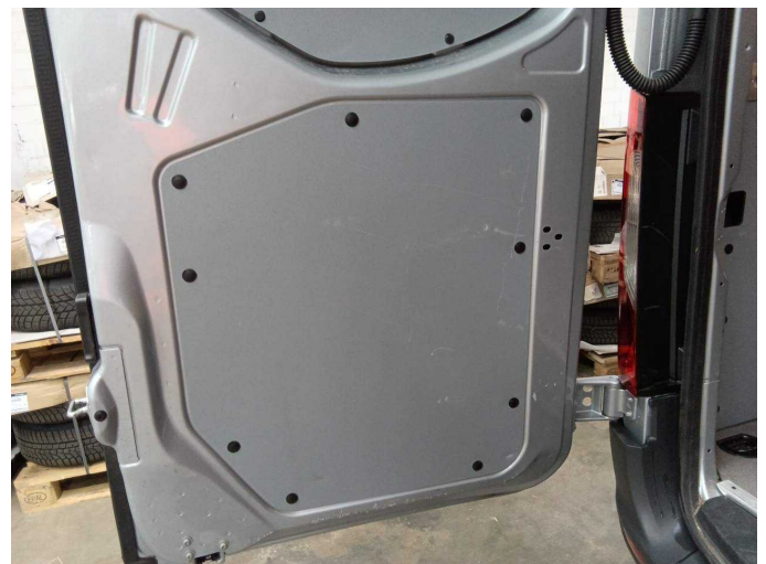
Damage 6: Trim / covers: Boot lining (Tür links unten) - Holes - Replace
