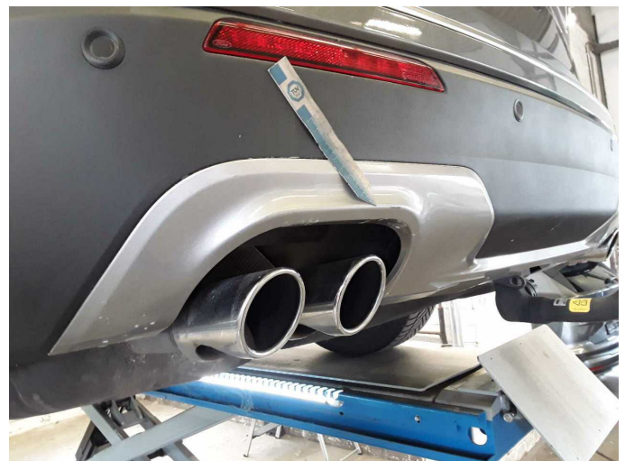
Damage 1: Rear bumper: Spoiler - Scratch(es) - Smart repair
