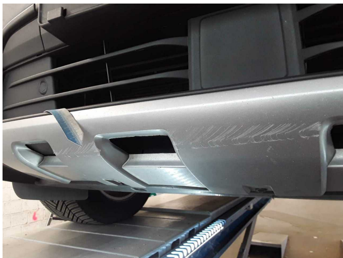
Damage 2: Front bumper: Spoiler - Scratched - Smart repair
