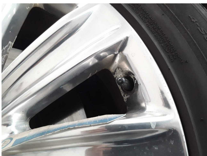
Damage 4: Wheel / tyres: Alloy rim - front right side (Oxidiert) - Worn - Loss in value
