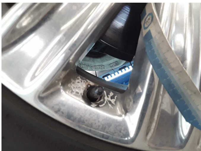
Damage 7: Wheel / tyres: Alloy rim - front left side (Oxidiert) - Worn - Loss in value
