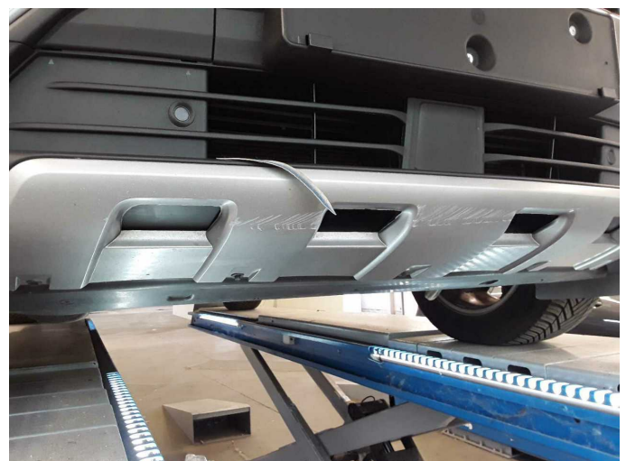
Damage 2: Front bumper: Spoiler - Scratched - Smart repair
