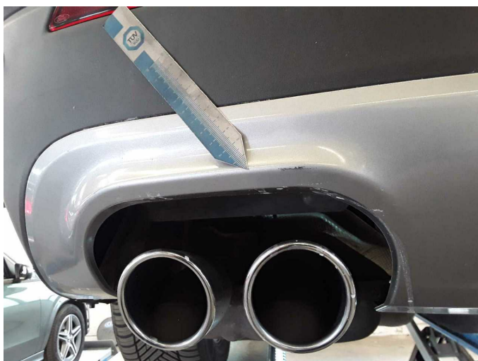
Damage 1: Rear bumper: Spoiler - Scratch(es) - Smart repair
