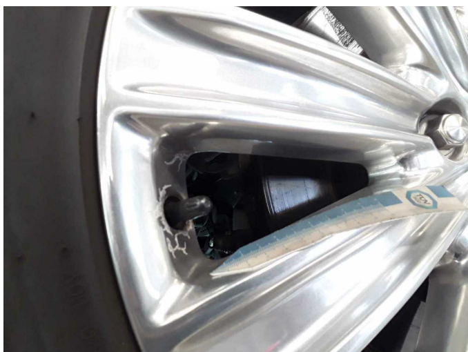
Damage 6: Wheel / tyres: Alloy rim - rear left side (Oxidiert) - Worn - Loss in value
