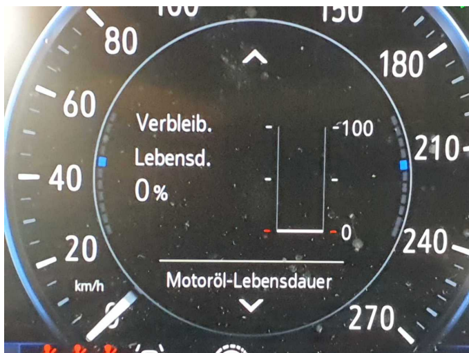
Damage 7: Misc.: Inspection / maintenance - Due - Replace
