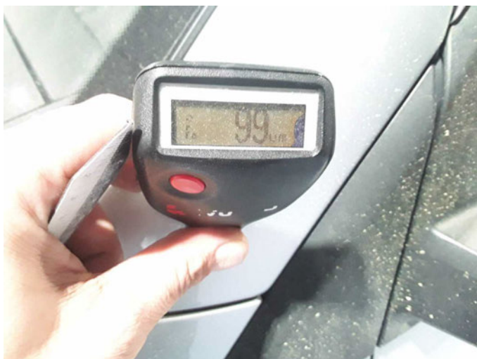
Dachholm links: 99 \mu\text{m}
