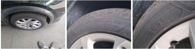
Tyre RR, Out of tolerance, Replace
