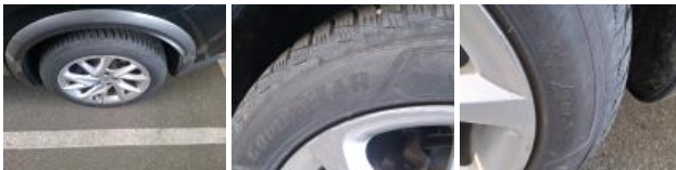
Tyre FL, Out of tolerance, Replace
