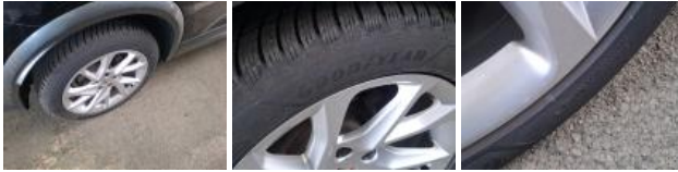
Tyre RL, Out of tolerance, Replace
