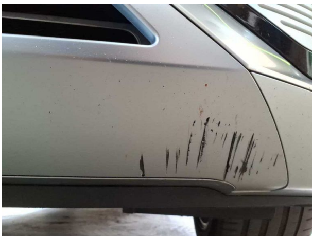
Damage #10: Front bumper: Spoiler - Scratched - Replace
