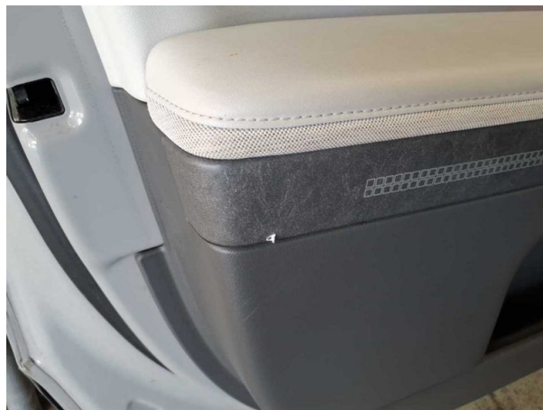
Damage #1: Trim / covers: Door trim - front left side - Scratch... - Smart repair
