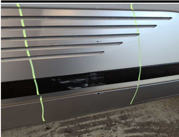
Damage #7: Door - front right side: Brightware - lower - Scratches... Replace
