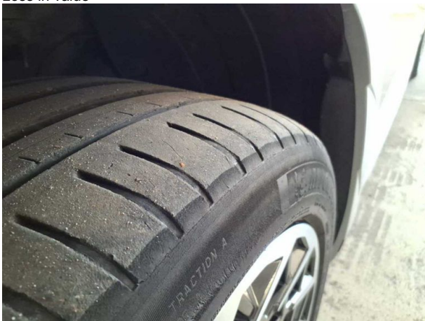
Damage #5: Measurement: Undercarriage - Malposition - Diagnosed and repair if necessary
