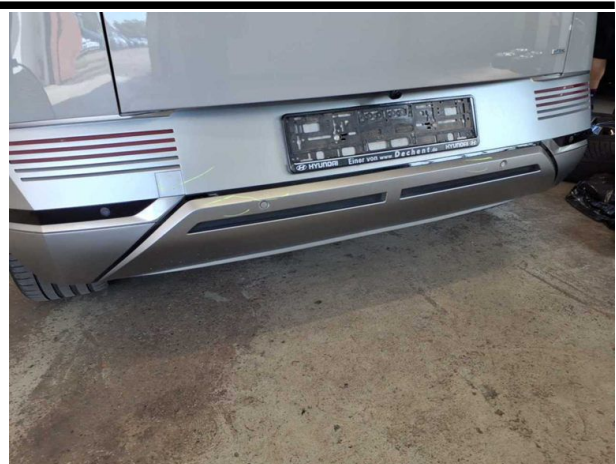
Damage #8: Rear bumper: Spoiler - Scratched - Repair and paint
