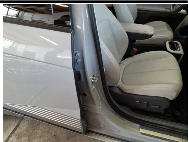
Damage #11: Sill - right side: Sill - Dent / paintcoat damage - Repair and paint
