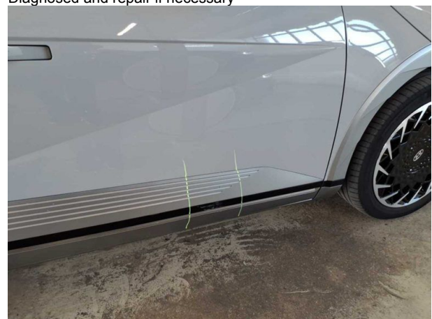
Damage #7: Door - front right side: Brightware - lower - Scratched - Replace
