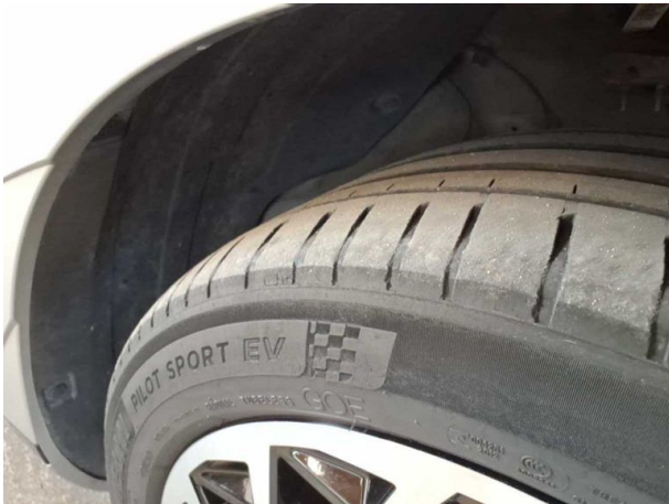
Damage #9: Wheel / tyres: Tyre - front - Worn - Replace
