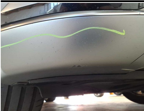
Damage #10: Front bumper: Spoiler - Scratched - Replace
