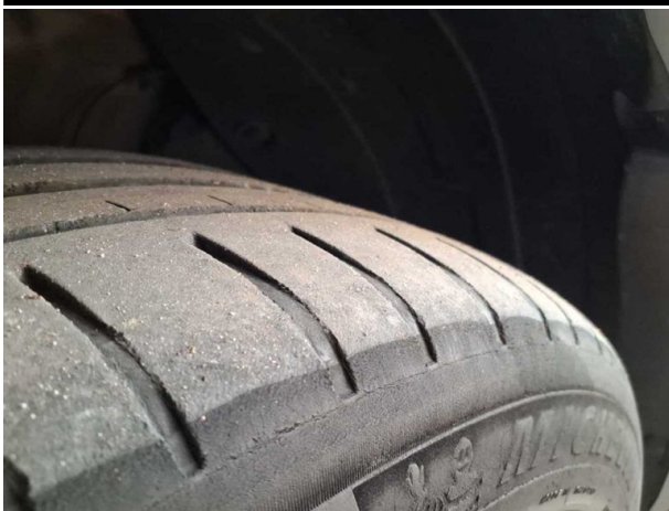
Damage #9: Wheel / tyres: Tyre - front - Worn - Replace
