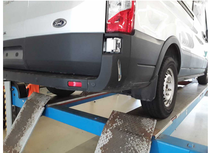
Damage 14: Rear bumper: Bumper - rear right side - Broken / torn - Replace
