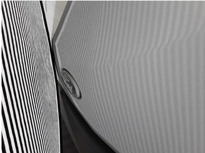
Damage 13: Boot lid / rear door: Rear door - right side - dent(s) - Smart repair
