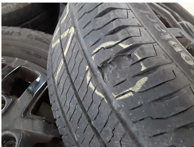
Damage 11: 2nd wheel set: 1 tyre - Broken / torn - Replace
