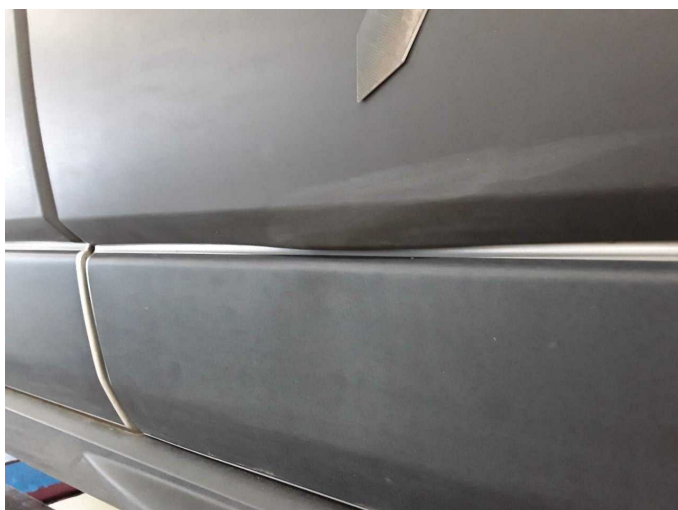
Damage 6: Sliding door, right: Protection strip - Deformed - Replace
