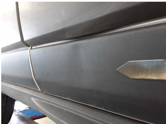
Damage 5: Sliding door, right: Sliding door with glass panel - dent(s) - Smart repair
