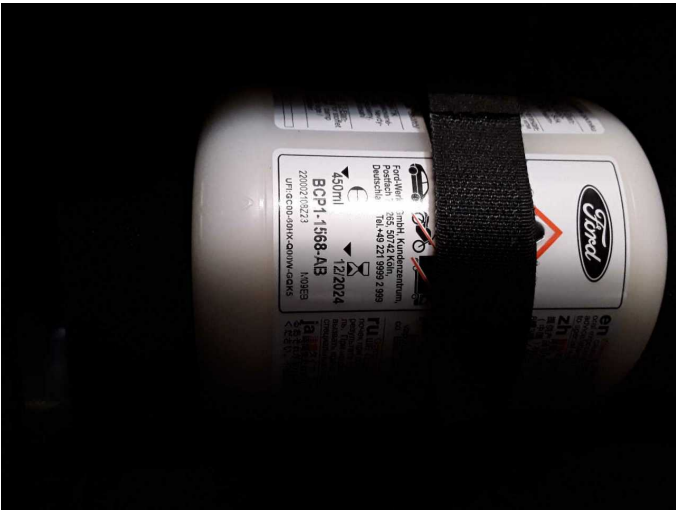
Damage 1: Equipment: Tirefit filler - Expired - Replace
