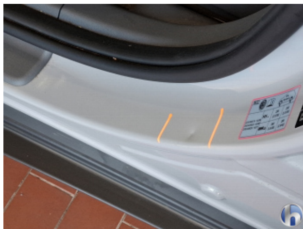
3. Türeinstieg Vorne - Links 1 Delle - Smart Repair
