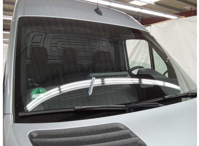
Damage 9: Vehicle glazing: Windscreen (kein Staubschutz) - Broken / torn - repair according to calculation
