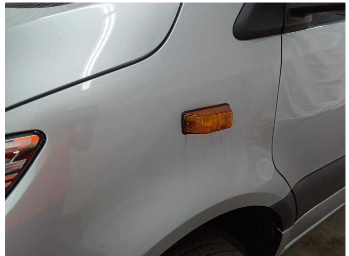
Damage 5: Indicator - front: Indicator lamp - front left side (Wassereintritt) - Leaking - Replace
