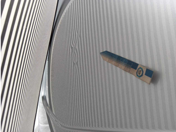
Damage 8: Boot lid / rear door: Rear door - left side (4) - dent(s) - Smooth repair work
