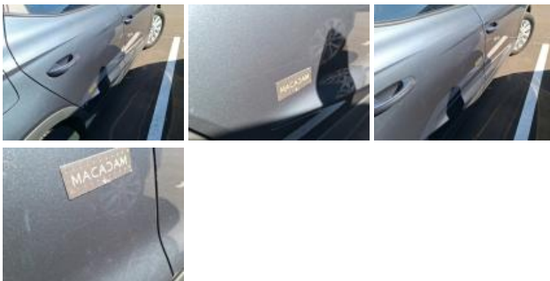
Door FR, Scratch(es), Repair and paint (complete)
