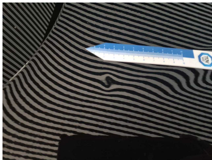
Damage 11: Bonnet: Bonnet (+ Steinschläge) - dent(s) - Paint
