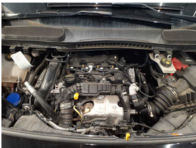
Missing part 1: Engine: Engine cover - Missing - Replace
