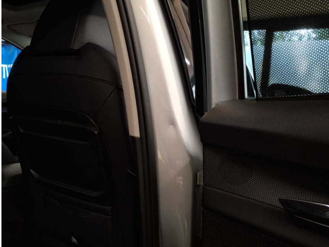
Damage 2: Body: B-pillar - right side - dent(s) - Smooth repair work
