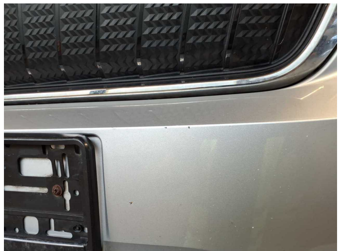
Damage 4: Front bumper: Front bumper (+ Kratzer) - Stone chips - Paint
