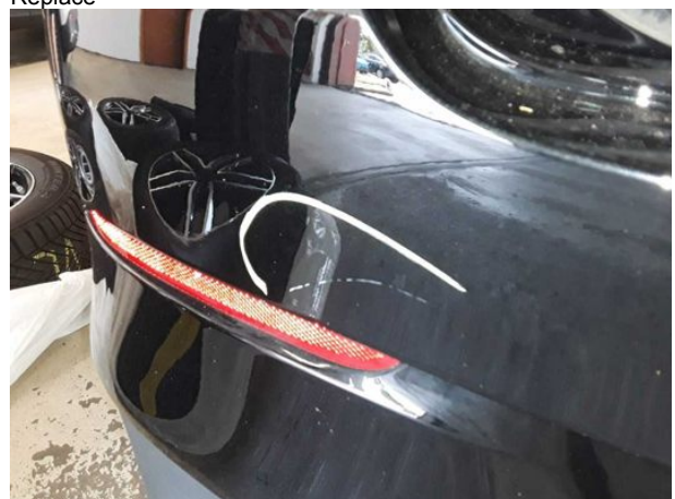
Damage #13: Rear bumper: Rear bumper - Damaged - Replace
