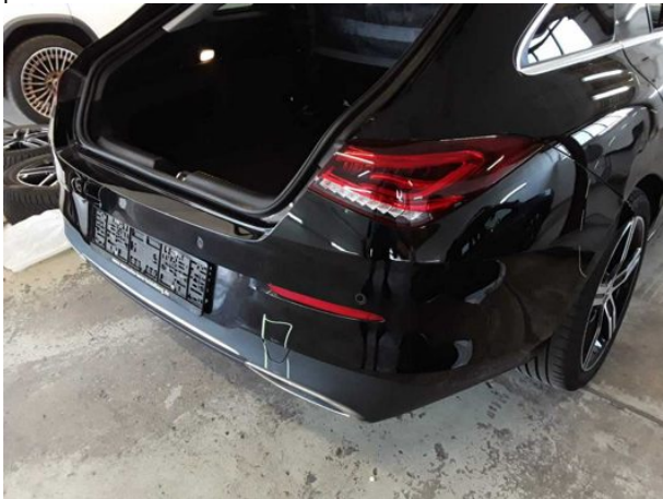
Damage #13: Rear bumper: Rear bumper - Damaged - Replace
