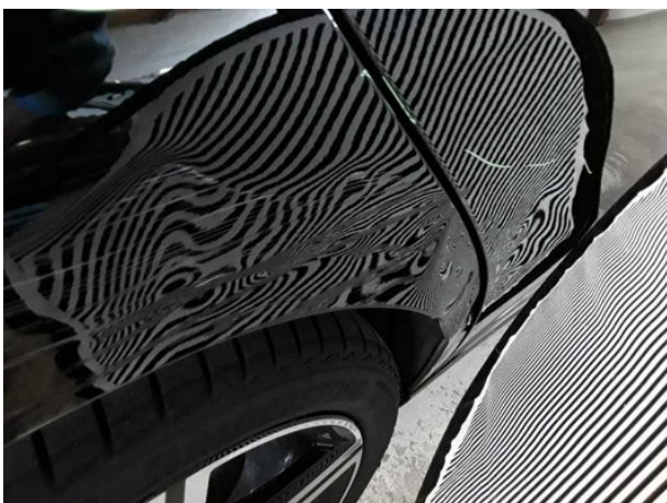
Damage #15: Side panel - rear right side: Side panel - Deformed - Replace
