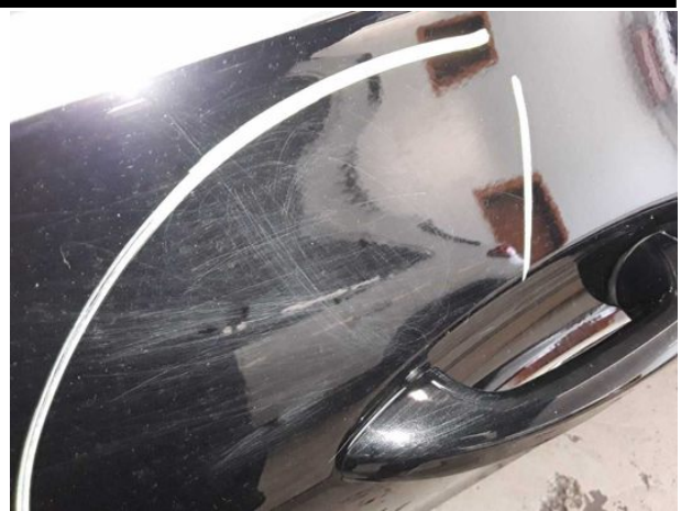
Damage #12: Door - front left side: Door - Scratched - Repair and paint
