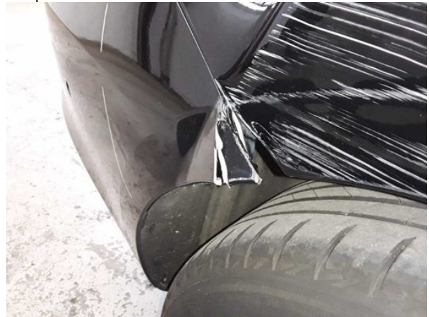
Damage #13: Rear bumper: Rear bumper - Damaged - Replace
