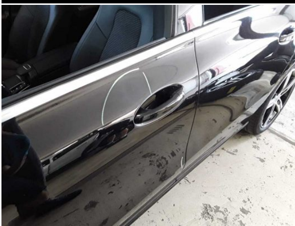
Damage #12: Door - front left side: Door - Scratched - Repair and paint
