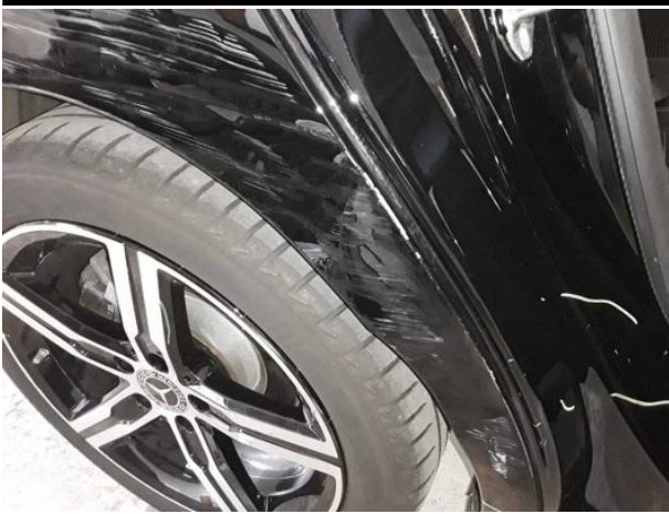
Damage #15: Side panel - rear right side: Side panel - Deformed - Replace
