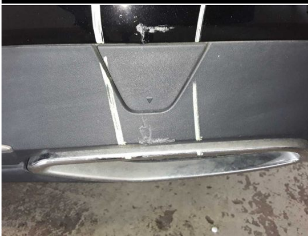
Damage #7: Rear bumper: Spoiler - Scratched - Replace
