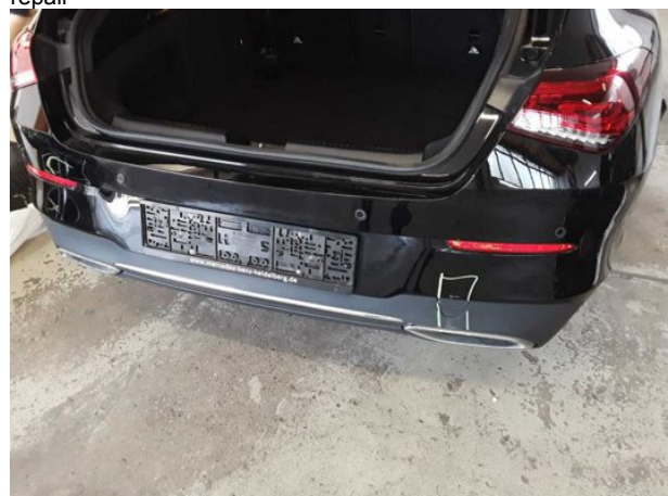
Damage #7: Rear bumper: Spoiler - Scratched - Replace
