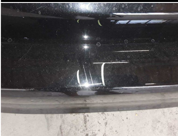
Damage #4: Rear bumper: Rear bumper - Scratched - Paint
