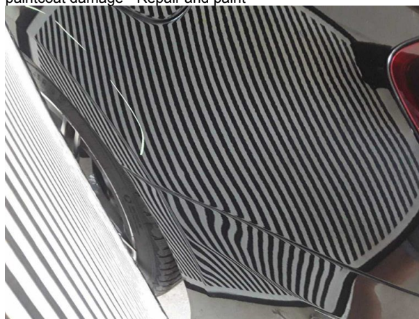
Damage #7: Side panel - rear left side: Side panel - Dent / paintcoat damage - Repair and paint
