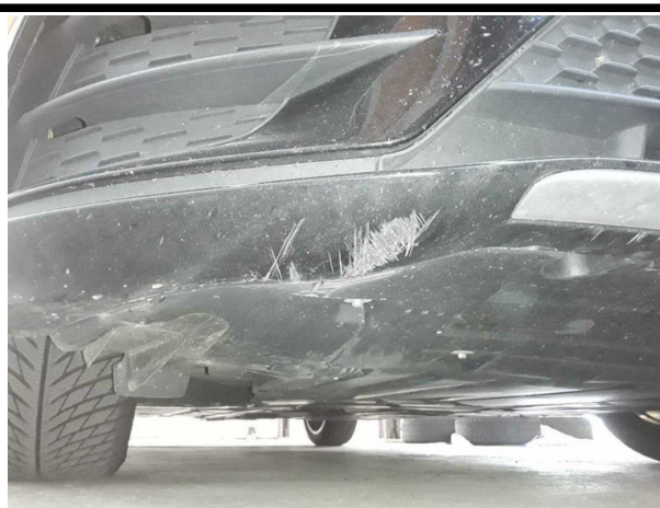
Damage #6: Front bumper: Front bumper - Scratched - Paint
