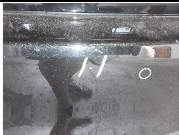
Damage #4: Rear bumper: Rear bumper - Scratched - Paint
