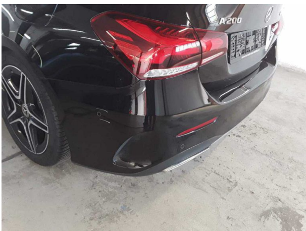
Damage #4: Rear bumper: Rear bumper - Scratched - Paint
