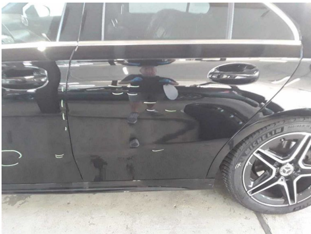
Damage #5: Door - rear left side: Door - Scratched - Paint
