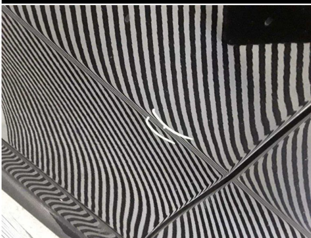
Damage #9: Door - front left side: Door - Dent / paintcoat damage - Repair and paint
