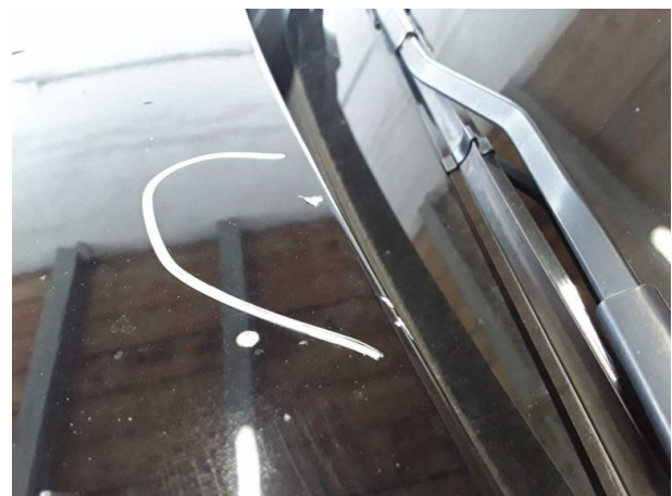
Damage #7: Bonnet: Bonnet - Scratch(es) - Paint
