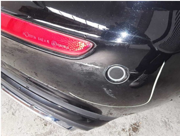
Damage #6: Rear bumper: Rear bumper - Scratched - Paint
