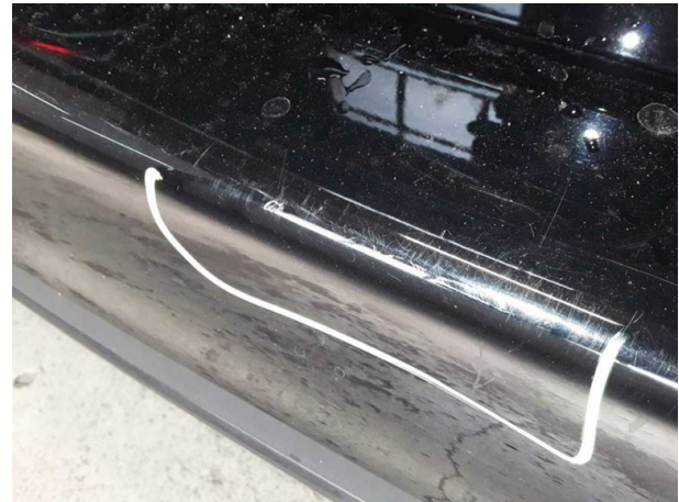
Damage #6: Rear bumper: Rear bumper - Scratched - Paint
