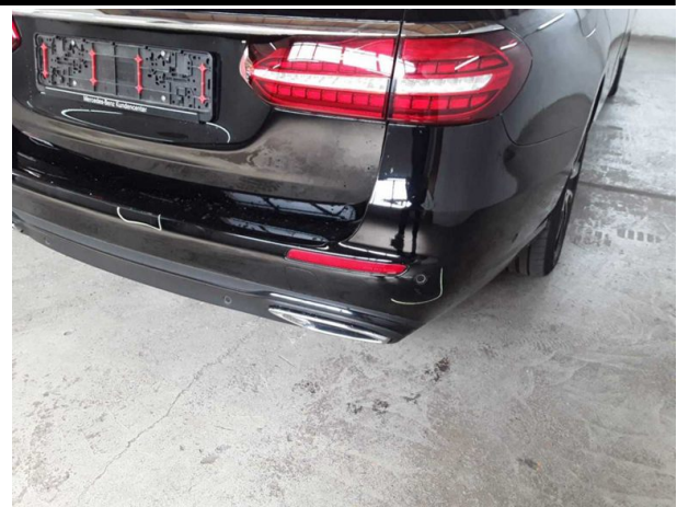
Damage #6: Rear bumper: Rear bumper - Scratched - Paint
