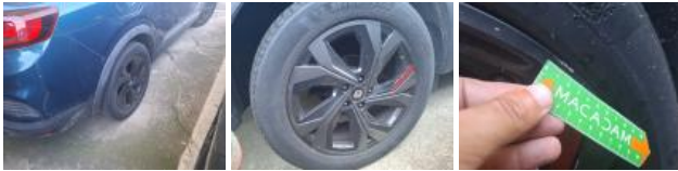
Tyre RR, Out of tolerance, Replace
