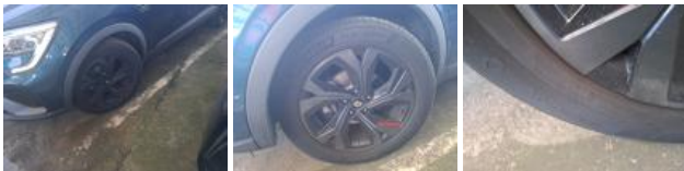
Tyre RL, Out of tolerance, Replace
