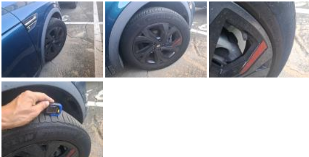
Tyre FL, Out of tolerance, Replace
