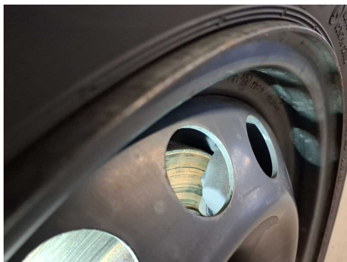
Damage 9: Braking system: Brake discs and brake pads - front (Tragbild mangelhaft, Rost) - Worn - Replace
