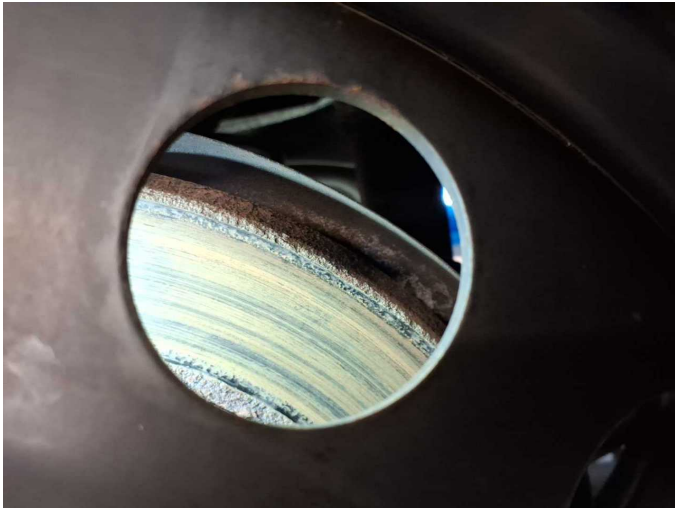
Damage 10: Braking system: Brake discs and pads - rear (Tragbild mangelhaft, Rost) - Worn - Replace
