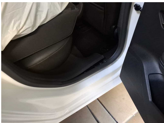
Damage 6: Trim / covers: Sill - front right side - Damaged - Replace
