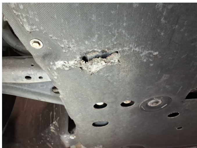
Damage 8: Body: Underbody panelling - Damaged - Replace
