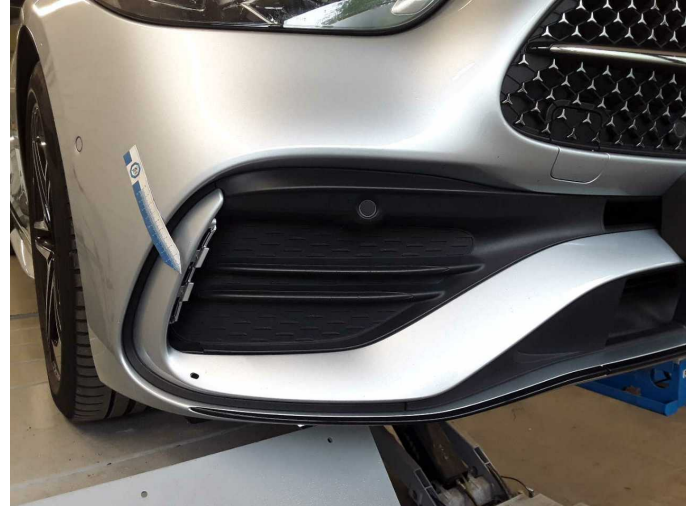
Damage 3: Front bumper: Cover bumper - front (Rechts) - Missing - Replace
