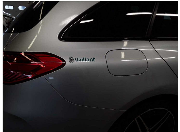
Damage 4: Body: Body - Glued / labelled - De-glue / neutralise
