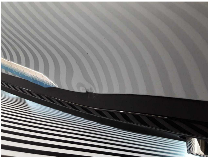
Damage 9: Rear bumper: Rear bumper - Damaged - repair according to calculation
