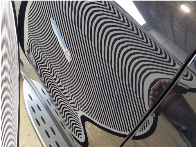
Damage 2: Door - rear right side: Door (Einschlüsse und wellig) - Unprofessionally repaired - Repair and paint
