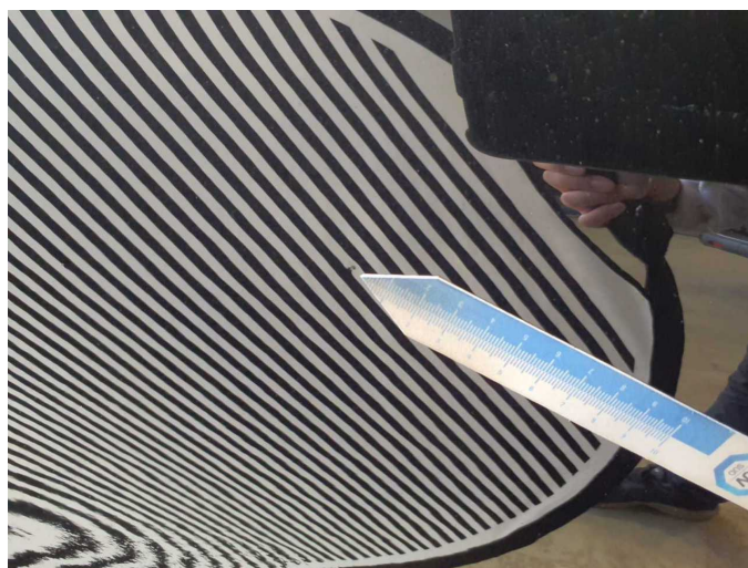
Damage 2: Door - rear right side: Door (Einschlüsse und wellig) - Unprofessionally repaired - Repair and paint
