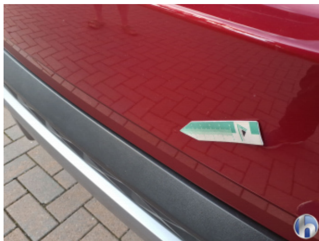
3. Heckklappe Kratzer - Smart Repair
