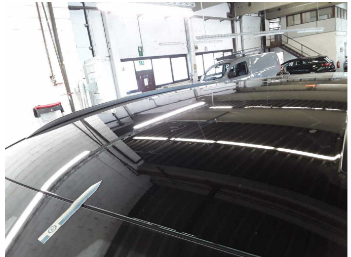
Damage 1: Roof: Roof - dent(s) - Smooth repair work
