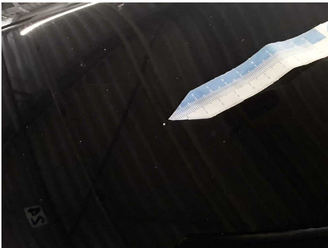
Damage 9: Bonnet: Bonnet - Stone chips - Paint
