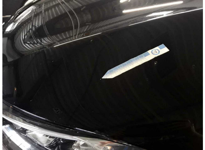
Damage 9: Bonnet: Bonnet - Stone chips - Paint
