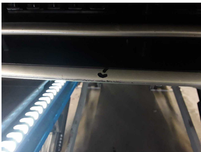
Damage 6: Front bumper: Spoiler (Zierleiste) - Scratched - Replace
