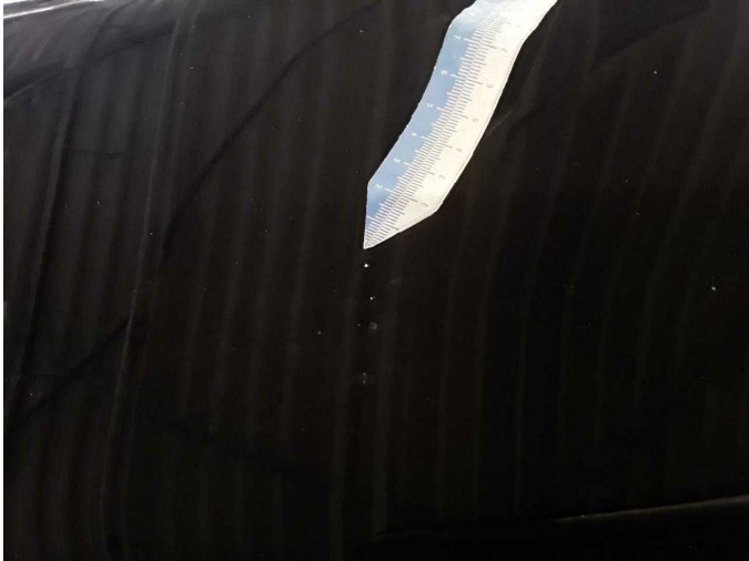
Damage 9: Bonnet: Bonnet - Stone chips - Paint
