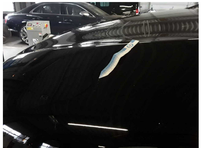
Damage 9: Bonnet: Bonnet - Stone chips - Paint
