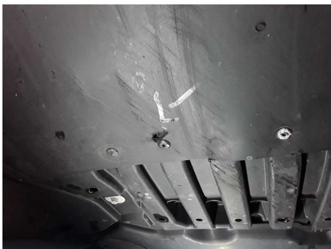
Damage 4: Body: Underbody panelling - Broken / torn - Replace
