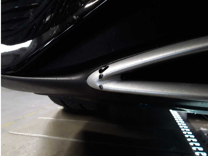
Damage 6: Front bumper: Spoiler (Zierleiste) - Scratched - Replace
