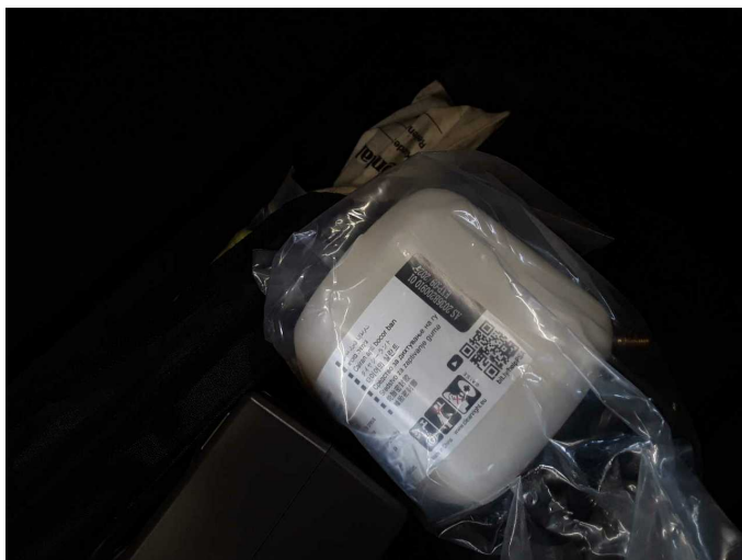
Damage 1: Equipment: Tirefit filler - Expired - Replace
