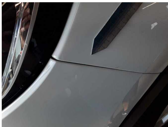
Damage 5: Front bumper: Front bumper - Malposition - Set / adjust
