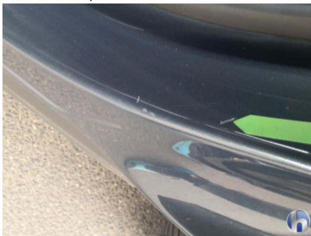
5. Schweller - Links Kratzer - Smart Repair
