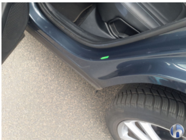
5. Schweller - Links Kratzer - Smart Repair
