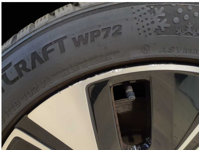
Damage 2: Wheel / tyres: Alloy rim - front right side - Scratch(es) - Replace
