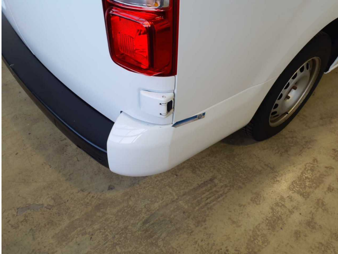
Damage 10: Rear bumper: Bumper - rear right side - Scratch(es) - Smart repair
