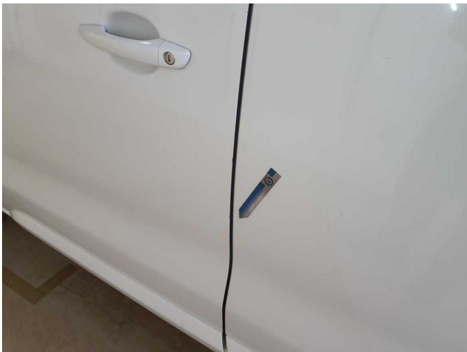
Damage 11: Door - front left side: Door - Scratch(es) - Smart repair
