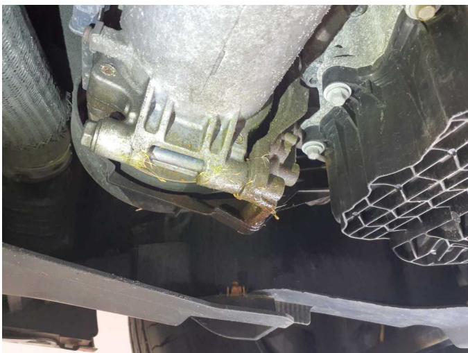
Damage 12: Engine: Engine - Leaking - Perform diagnosis
