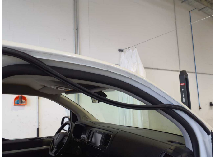
Damage 4: Door - front right side: Door seal - Loose - Un- / install
