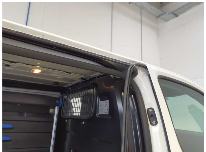
Damage 13: Sliding door, right: Door seal - Broken / torn - Replace
