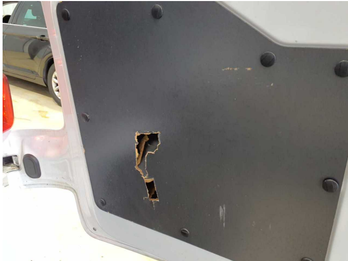
Damage 17: Trim / covers: Door trim - rear right side - Broken / torn - Replace
