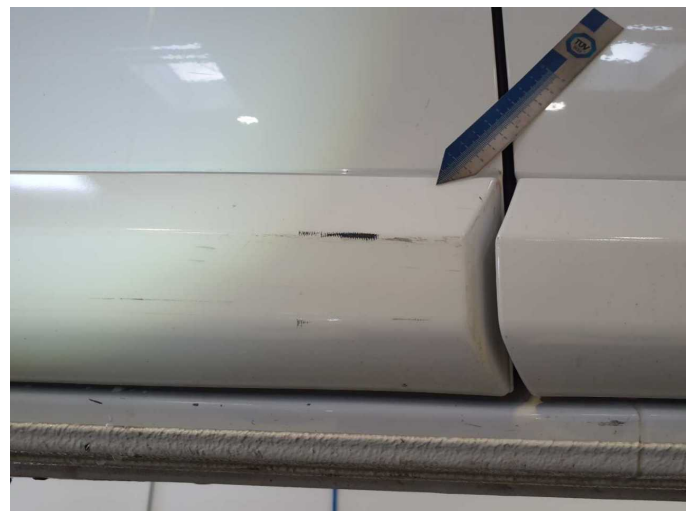
Damage 16: Door - rear right side: Brightware - lower - Scratch(es) - Paint
