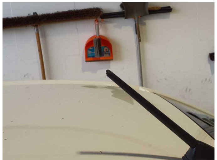
Damage 2: Roof: Stub aerial - Broken / torn - Replace
