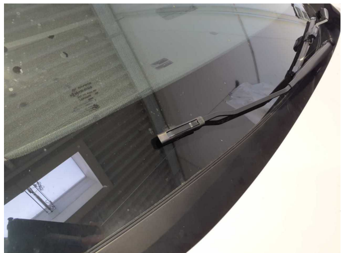
Damage 6: Screen cleaning: Wiper blades - front - Missing - Replace
