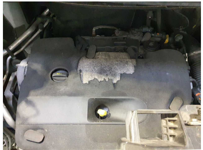
Damage 15: Engine: Engine cover - Damage caused by marten / rodent - Replace
