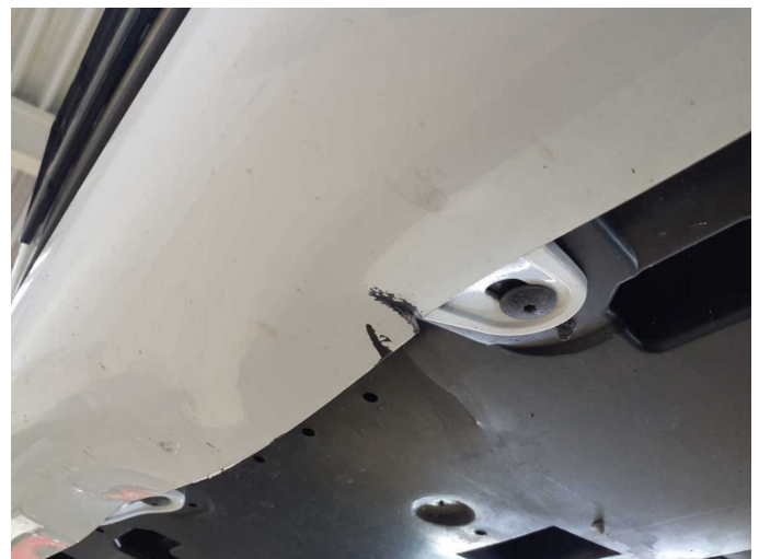
Damage 18: Front bumper: Front bumper - Broken / torn - repair according to calculation
