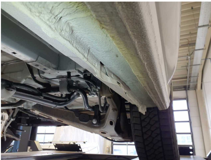
Damage 14: Sill - left side: Sill - dent(s) - Smart repair
