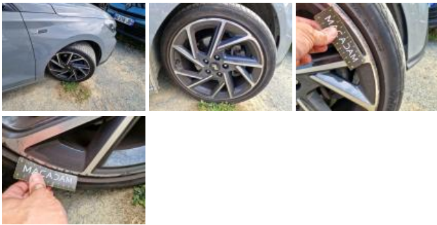
Tyre FL, Out of tolerance, Replace
