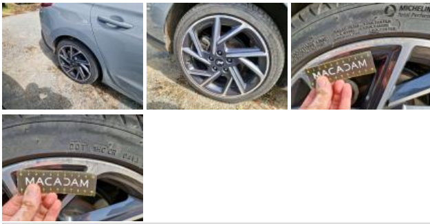
Tyre FR, Out of tolerance, Replace
