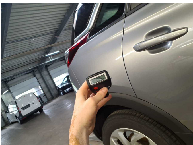
Repainting 2: Side panel - rear right side
