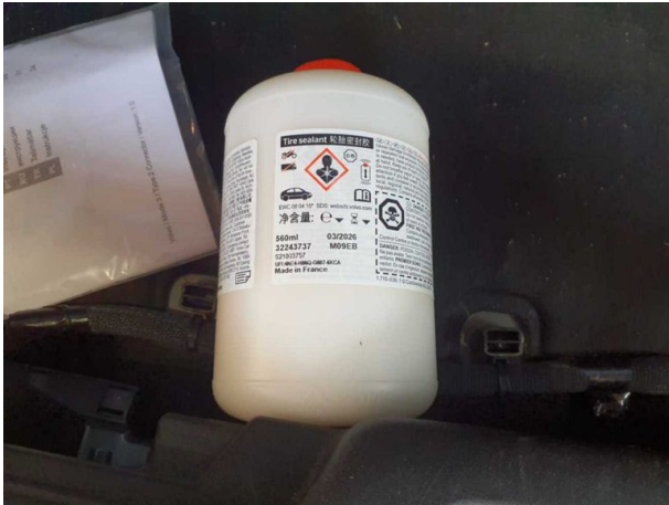
Damage #1: Equipment: Tirefit filler - Expired - Replace
