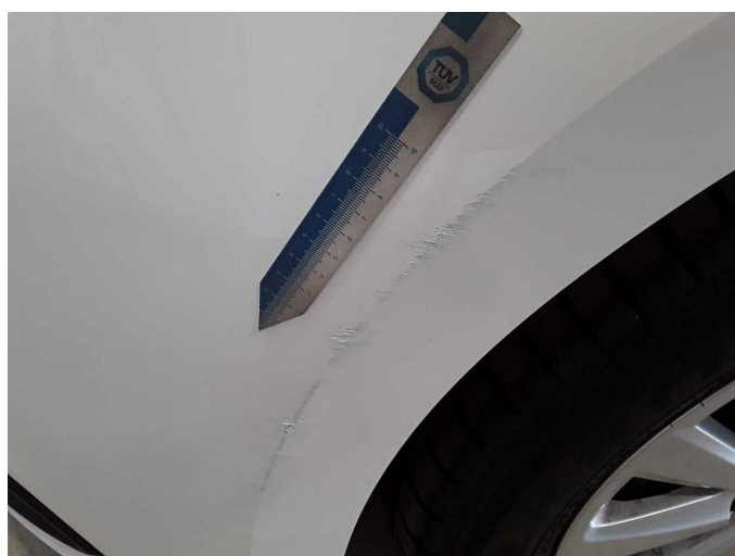
Damage 4: Front bumper: Front bumper - Scratch(es) - Paint
