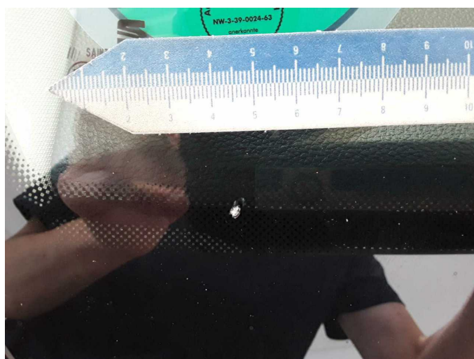
Damage 5: Vehicle glazing: Windscreen - Broken / torn - Replace
