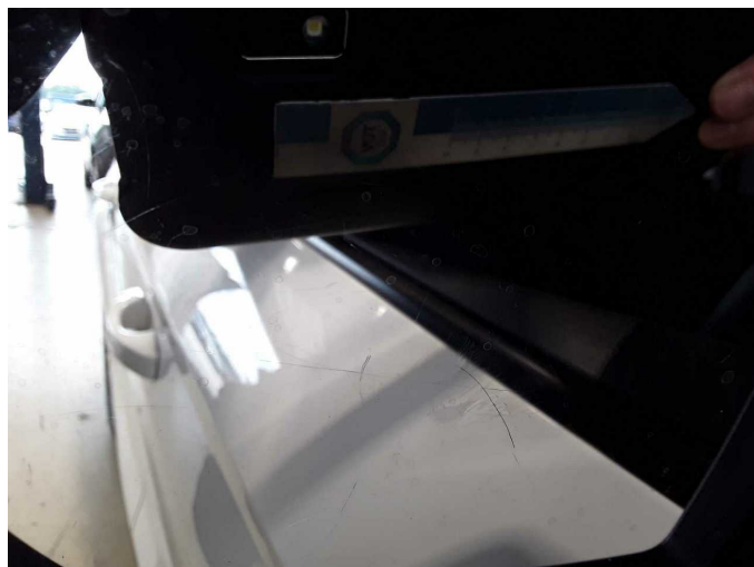
Damage 3: Wing mirror - left side: Mirror glass - Scratch(es) - Replace
