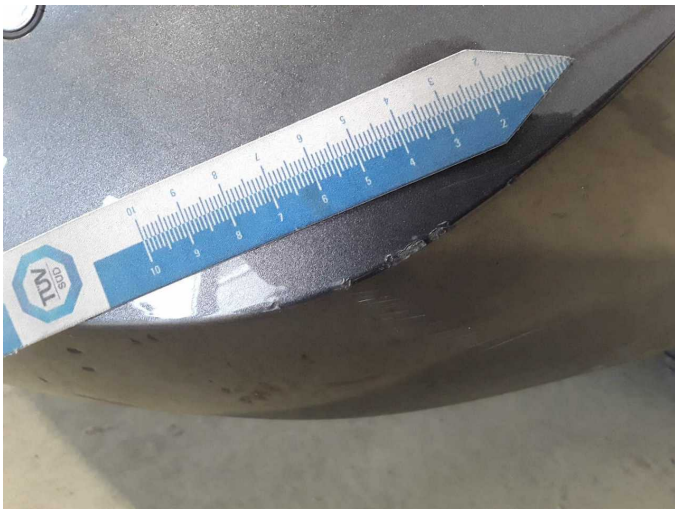
Damage 6: Rear bumper: Rear bumper - Scratch(es) - Paint
