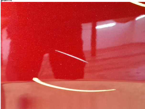
Damage #6: Side panel - rear right side: Side panel - Scratched - Repair and paint
