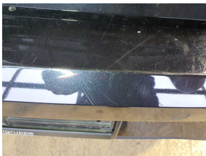
Damage 13: Rear bumper: Rear bumper - Scratch(es) - Paint
