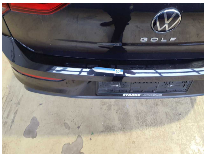
Damage 13: Rear bumper: Rear bumper - Scratch(es) - Paint
