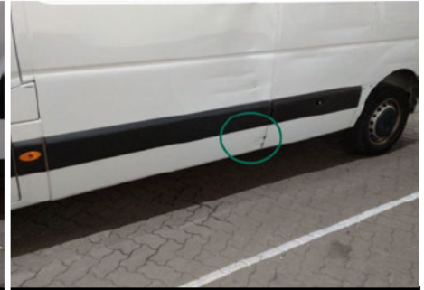
Schweller / Vorne Links / Delle
