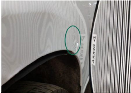
Kotflügel / Vorne Links / Delle
