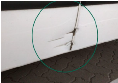
Schweller / Vorne Links / Delle
