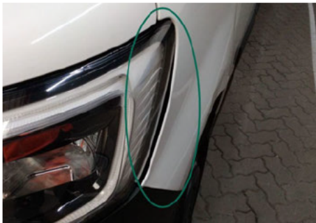
Kotflügel / Vorne Links / Delle
