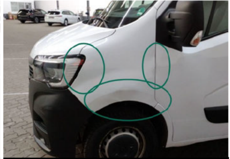
Kotflügel / Vorne Links / Delle
