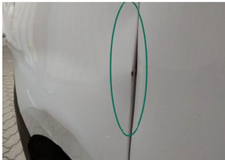
Kotflügel / Vorne Links / Delle
