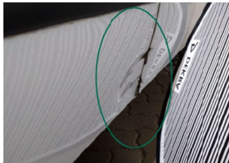
Schweller / Vorne Links / Delle
