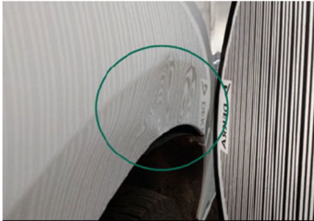
Kotflügel / Vorne Links / Delle
