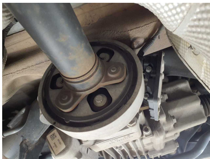
Damage 4: Drive train: Drive train (Harddiscs) - Porous / cracked - Replace
