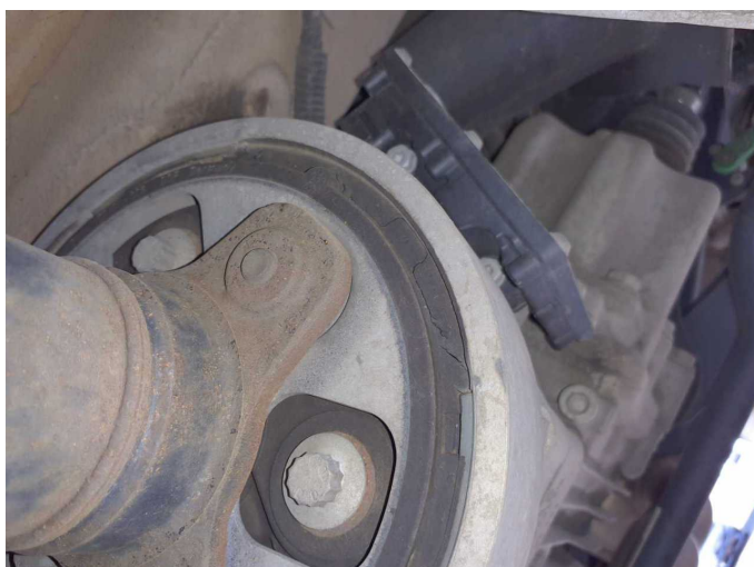
Damage 4: Drive train: Drive train (Harddiscscheibe) - Porous / cracked - Replace
