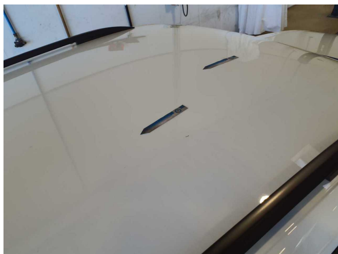
Damage 5: Roof: Roof - Damage by hail - Smooth repair work
