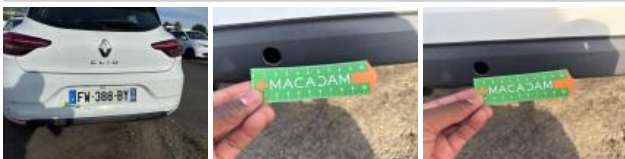
Parking sensor R, Missing, Replace
