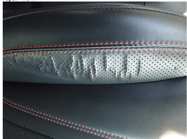
Damage #2: Seat - front: Seat cover - left side - Broken / torn - Replace
