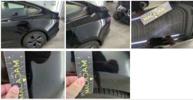
Door FL, Scratch(es), Repair and paint (complete)
