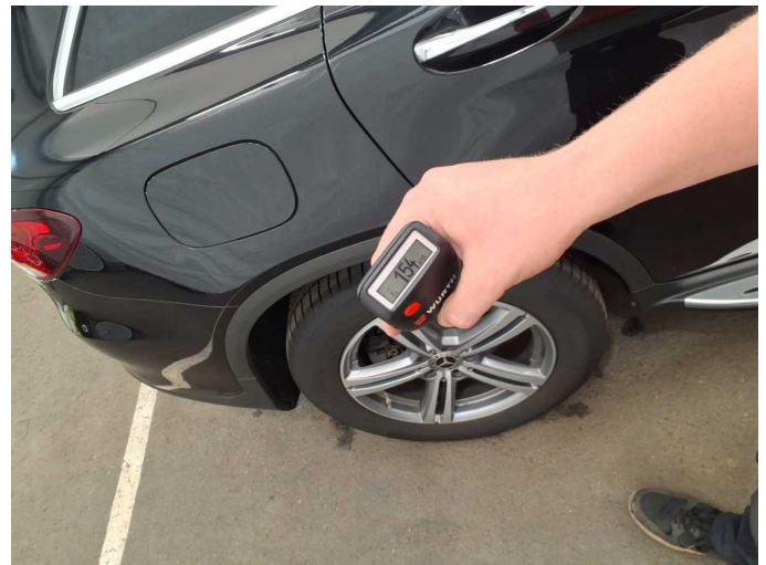
Repainting 1: Side panel - rear right side
