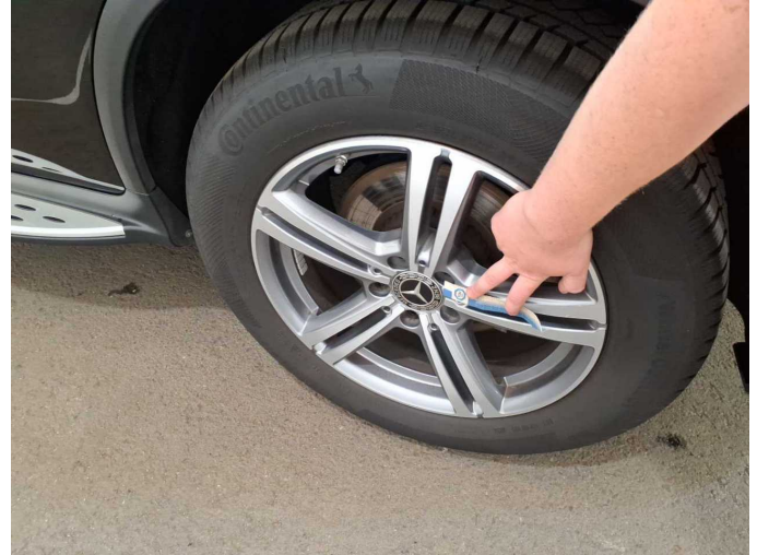
Damage 1: Wheel / tyres: Wheel rim - rear left side - Scratch(es) - Loss in value
