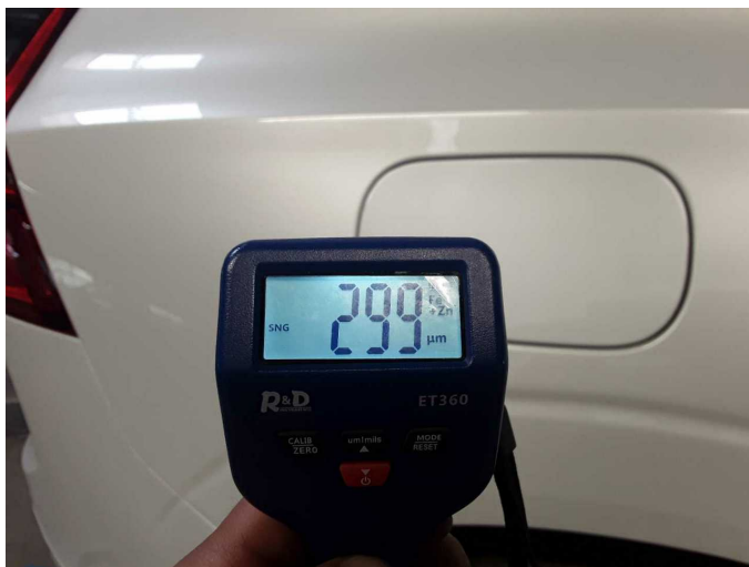
Side panel - rear right side: 299 µm
