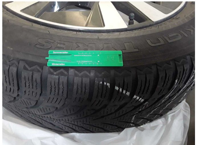
Damage 5: 2nd wheel set: 2 tyres (3mm) - Does not meet the leasing specifications - Replace
